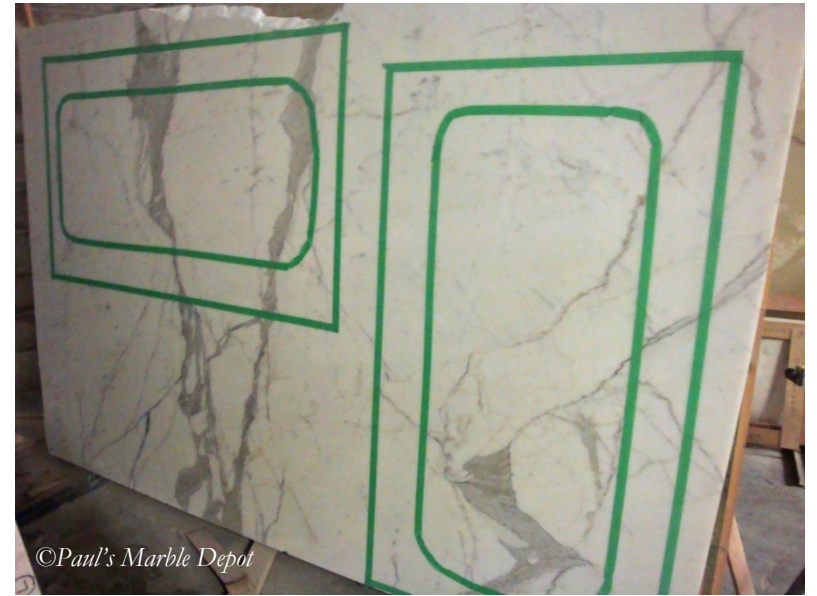
Template laid out on slab
